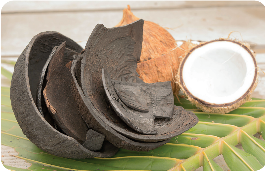
Activated carbons are used to absorb impurities during bleaching of edible oils and are commonly made from coconut shell, coal and wood
